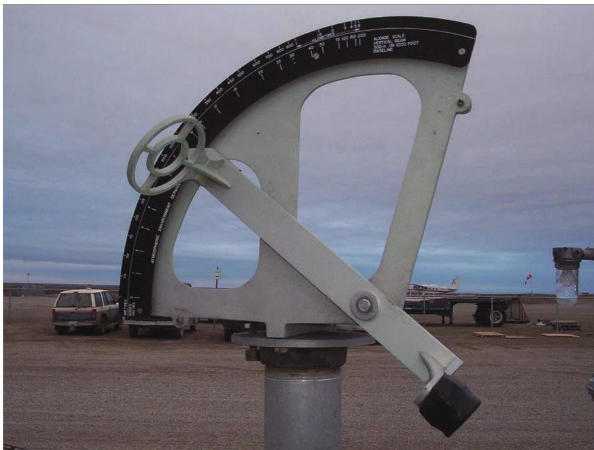
Figure 12.2 Finding the height of the cloud base using an alidade
