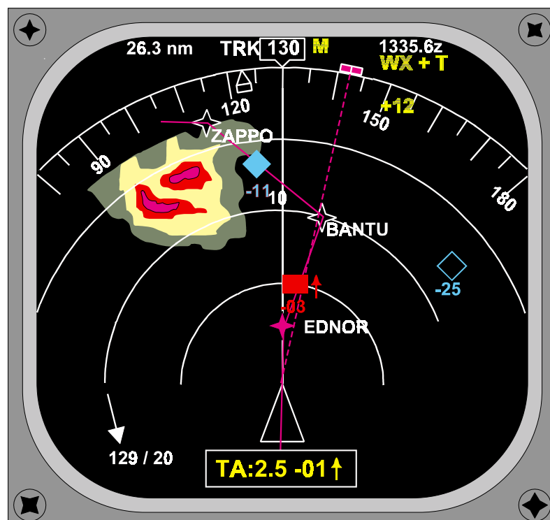
Figure 4.7a Navigation Display in MAP Mode Showing TCAS
